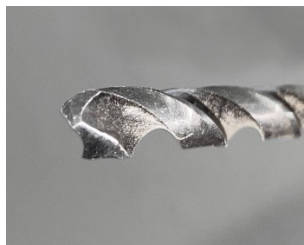
Pitted drill surface after repeated use
